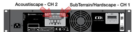
5. Attach the included RCA wires to the two phoenix connectors as shown in the illustration below. Make sure to match the colored wires in the correct order
