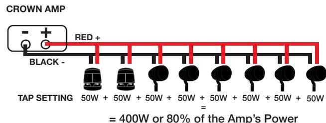
**NOTE:** If using 70V, the Acousticscape speakers MUST be set to the proper TAP setting prior to connecting it to the amplifier. The speaker will blow if set to 8Ω and will not be covered by warranty. The higher the TAP setting the more power it will receive from the amplifier and the louder the speaker will go. The TAP settings gives the listener greater flexibility for layout design. It also allows each speaker to be tapped at different levels creating an even sound stage.
