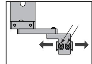
3) If up/down needs adjusting, reposition slotted screws on block "C".
