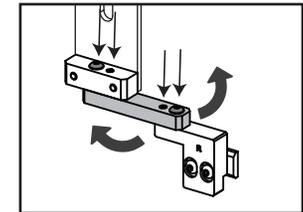
2) If side/side needs adjusting, loosen slotted screws on both "C" blocks, taking care not to let either end of the soundbar rise or lower before retightening.
