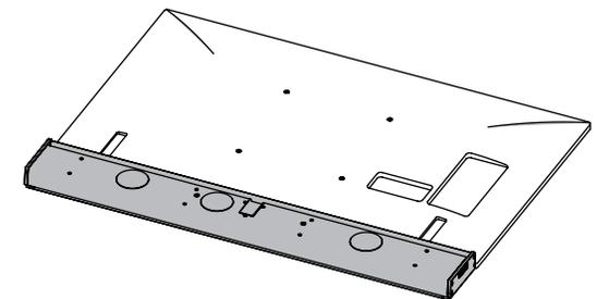
2) To determine which Vertical Bars to use, place a bar even with the edge of the TV where the soundbar will be mounted. The slot in the bar should cover both VESA holes, but not extend beyond the TV.
