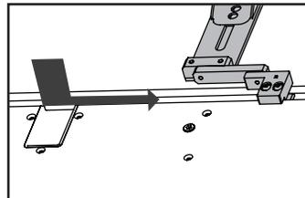
7) Align the soundbar to the TV. Place the Vertical Bar over the VESA mounting holes in the TV. The swivel bracket assemblies should be oriented outwards. Lay the TV mount over the top of the Vertical Bars and thread (but do not tighten) the TV mount hardware into place.
