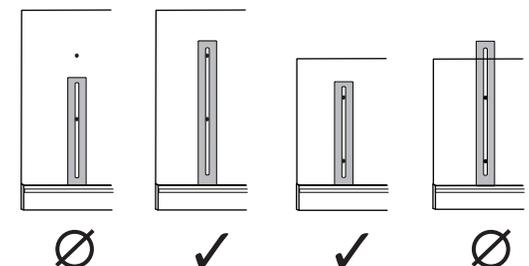
3) Attach the swivel bracket to the selected vertical bars using the included flat head screws. The beveled edges of block "A" should face away from the vertical bar.
