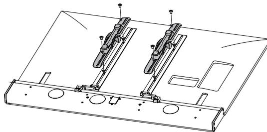
8) Loosely tighten the mount hardware. Begin with the screws closest to the soundbar and work towards the TV mount. Keep the screw heads centered in their slots in block "C" for now.
