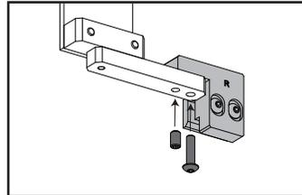
6) Install the right and left swivel brackets onto the soundbar. Loosen the screws in block "C" so that the ends are flush with the cleat. Insert the cleat at an angle into the channel, beginning at the center of the soundbar, and slide to the appropriate side. Repeat with the other side.
