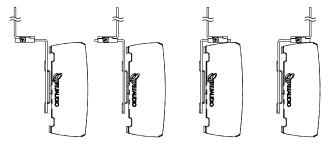
**Note:** You may need to loosen the screws in the lower part of the VERT bracket to allow the WIDE bracket tab to move freely.
