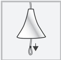
Thread the looped end of the cable through the top cap before attaching the carabiner
