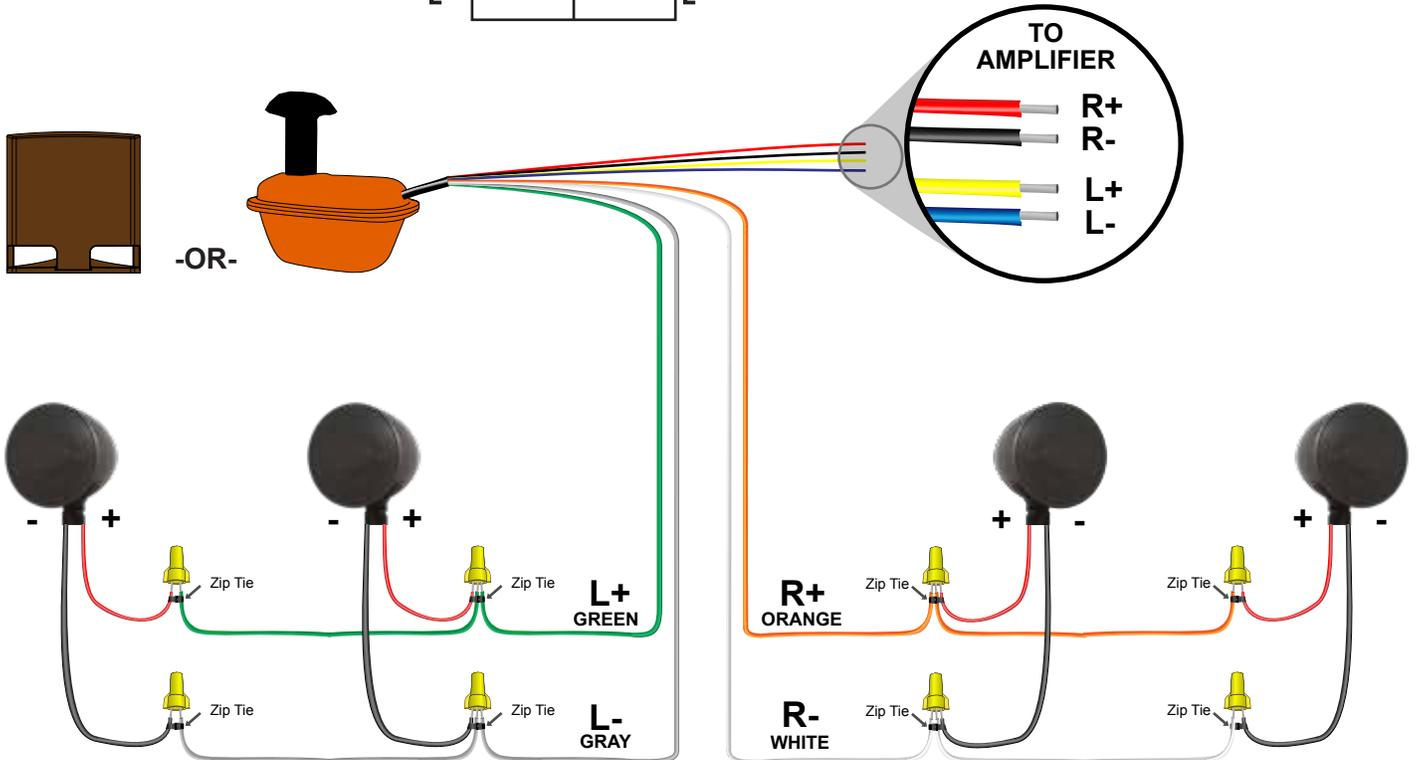
The UltraScape system **MUST** be wired as seen above. You cannot put more than two satellite speakers on each side. Doing so can damage your system.
