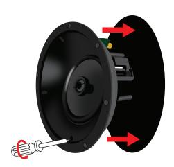
3. Place speaker into the hole with the drive angle pointing to the listening area. Tighten the dog ears to secure the speaker in place. Be sure to not over tighten the mounting screws.
